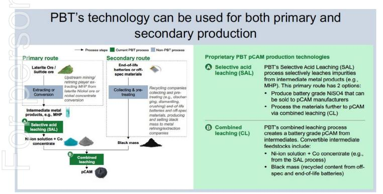
PBT's technology can also be used to recycle existing LIB materials creating a closed-loop lifecycle for these critical battery minerals. In September 2020, PBT acquired an existing refinery in Hagen, Germany, providing a base to demonstrate the commercial viability of PBT's technology. PBT is a publicly unlisted company. Further information on PBT can be found at *www.purebatterytech.com*
